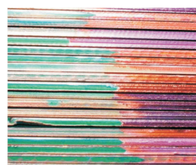
Figure 2. Multilayer PCBs.
